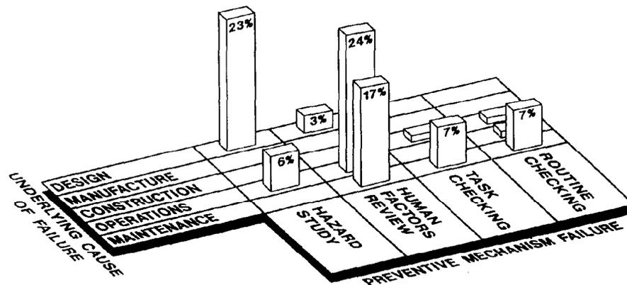
**Figure 1** Analysis of accident data: Major Accident Reporting System (MARS)<sup>11</sup>
